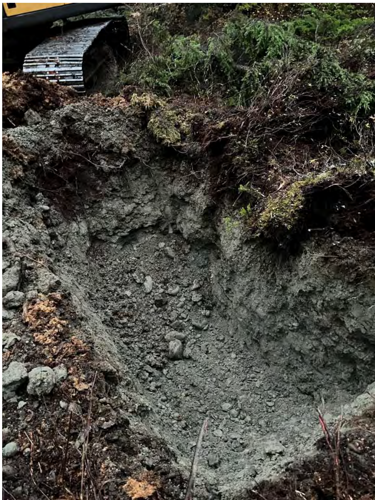
Photo A - 33: Test Pit TP33
